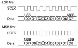
Fig. 5.8.6.1 Transfer data configuration using clock synchronous mode
